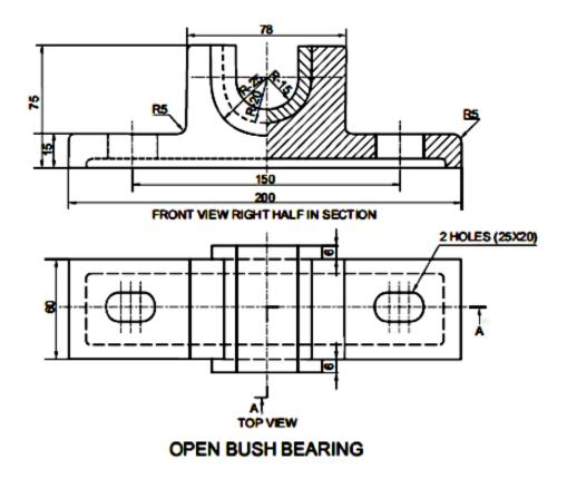
2. The Fig shows the assembly of Bushed Bearing. Dis-assemble the parts, and draw orthographic views of the following parts to scale 1:1, keeping same position:
